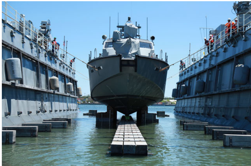
VIRGINIA BEACH, Va. (June 9, 2016) Dynamic (AFDL 6) Sailors stand by as dry-dock Dynamic, located at Joint Expeditionary Base Little Creek-Fort Story, begins to sink during the undocking of MK VI Patrol Boat 1202. (U.S. Navy photo by Shelby F.W. West/Released)
