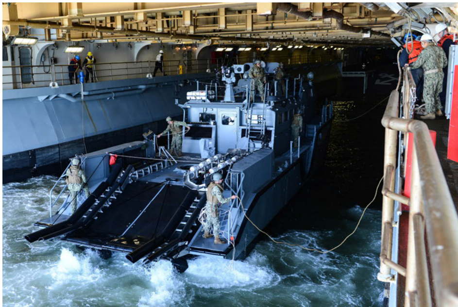
ATLANTIC OCEAN (May 1, 2016) Sailors moor a MK VI patrol boat attached to Coastal Riverine Squadron 4 (CRS4) during wet well operations onboard the multipurpose amphibious assault ship USS Bataan (LHD 5). The MK VI patrol boat is an 85-foot craft arranged with an ergonomically designed pilothouse, covered fly bridge, re-configurable main deck cabin and below-deck accommodations. Bataan is currently underway conducting routine qualifications in preparation for her future deployment. (U.S. Navy photo by Mass Communication Specialist 3rd Class Nicholas Frank Cottone/Released)
