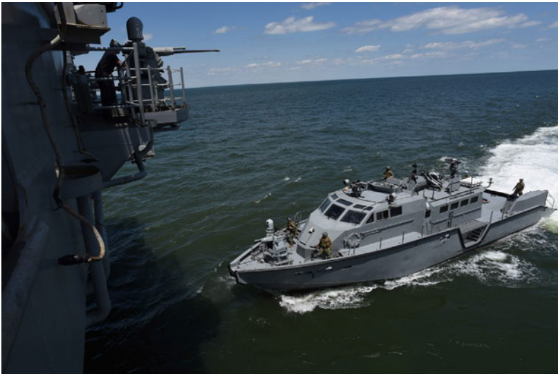
ATLANTIC OCEAN (May 1, 2016) A MK VI Patrol Boat attached to Coastal Riverine Squadron 4 (CRS 4) approaches the well deck of the amphibious assault ship USS Bataan (LHD 5) during wet well operations. The MK VI patrol boat is an 85-foot craft arranged with an ergonomically designed pilothouse, covered fly bridge, re-configurable main deck cabin and below-deck accommodations. Bataan is currently underway conducting routine qualifications in preparation for her future deployment. (U.S. Navy photo by Mass Communication Specialist 1st Class Julie Matyascik/Released)
