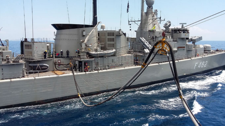
HS Axios (A 464) refuels the Hellenic Navy frigate HS Kountouriotis (F-462). (Hellenic Navy photo)
