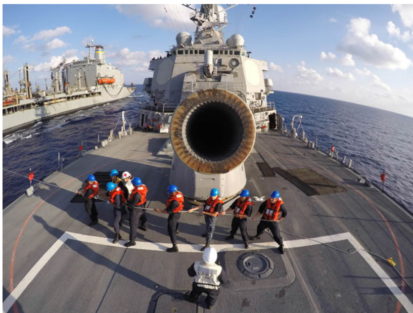
Sailors aboard USS Carney (DDG 64) hold the phone and distance line during a replenishment-at-sea with the Military Sealift Command fleet replenishment oiler USNS Big Horn (T-AO 198) in the Mediterranean Sea. Carney, an Arleigh Burke-class guided-missile destroyer, forward-deployed to Rota, Spain, is conducting a routine patrol in the U.S. 6th fleet area of operations in support of U.S. national security interests in Europe. (U.S. Navy photo by Mass Communication Specialist 3rd Class Weston Jones/Released)
