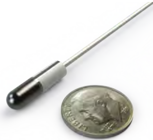
YES Sensor packaged in standalone probe configuration with size comparison to a US dime. Copyright Innoveering 2021
