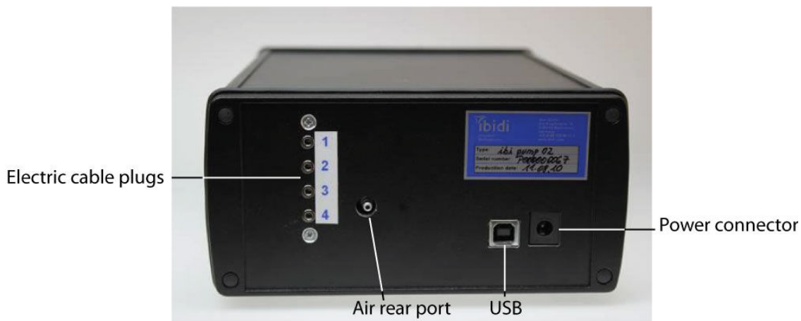
Figure 3: Rear view of the ibidi Pump with air rear port, connections for the USB, power supply port, and electrical cables ports to the Fluidic Units.
