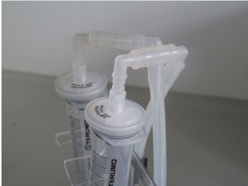
Figure 51: Cross the tubing on top of the reservoirs to test if the problem is with the Perfusion Set or in the valve block (valve 1).
