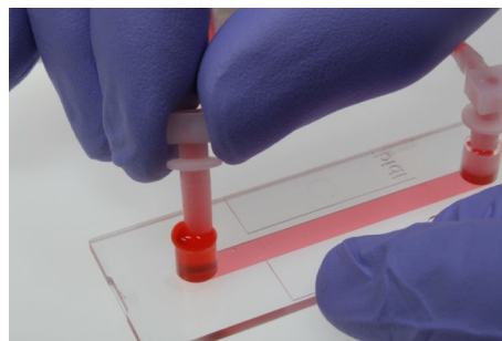
Figure 32: Connect the second Luer adapter to the \mu -Slide.
