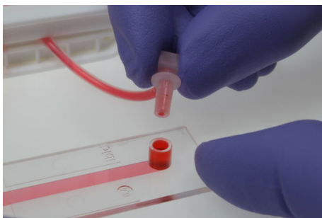
Figure 31: Fill the reservoir before connecting to the Luer adapter.
