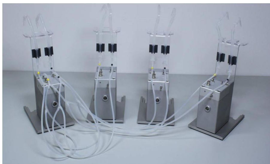
Figure 38: Oscillatory flow setup with four Fluidic Units (one master and three slaves).
