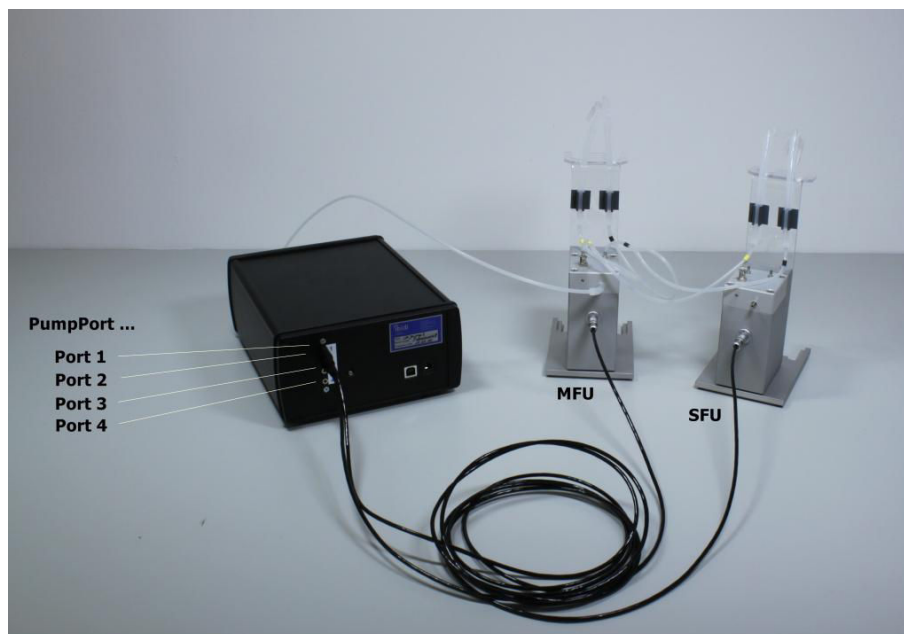
Figure 36: Oscillatory flow setup with two Fluidic Units (one master and one slave).
