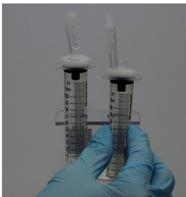
Figure 22: Squeeze the reservoirs for insertion into the holder.
