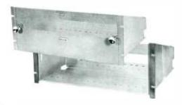
Used for rack or multiple mounting of plug-in units. Requires only 7" x 19" rack space. Front is ventilated by top half being perforated and is instantly removable to allow removing amplifiers from the front, or making gain adjustments. The BA-20 or BA-21 bases with receptacle, listed below, fasten to the bottom of the panel and shelf assembly. Depth is 13\(^3\kgamma\)". Finish medium gloss gray. Weight 10 lbs.
