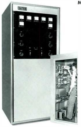
Fully FCC type approved, the Gates BC-250GY is the most widely used 250 watt AM broadcast transmitter and has a world-wide reputation for long trouble-free service. It consists of three audio frequency stages with provision for 2 crystals in temperature controlled ovens. The Type 813 RF driver provides an abundance of drive and long tube life. A pair of Type 810 single ended power amplifiers feed an output coupling network that will match specified impedances from 30 to 300 ohms.
