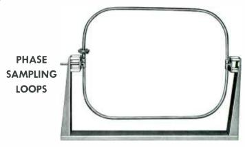
M-3283: This model especially applicable where high current ratios are to be sampled. May be rotated so that phase monitor amplitude values are nearly equal. Electrostatically shielded and insulated from tower. May be used with or without isolation coil at base of tower. Coil is single loop of %" coaxial cable, heavily insulated from base frame. Matches either 50 or 70 ohm line. Size: 48" wide, 32" high. Sompling Loop
