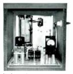
A fully weatherproof coupler for series feed antennas to handle 1250 watts or less and at 100% modulation. Meter shorting switch is provided in antenna circuit to eliminate damage to meter during electrical disturbances. Antenna meter may be observed through glass porthole, Coil is silver plated, having generous inductance for arrangement in a full Tee network along with the fixed mica capacitors supplied. Extra room is provided in the cabinet for either
