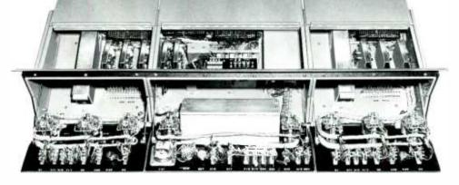
mounted in sturdy cast aluminum housings with interconnecting cables and plugs.
