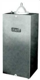
Model M-5178: Series feed, provides all coil capacitance to provide full Tee network. Constructed in non-weatherproof steel cabinet, front removable. Size: 21" high, 10" wide, 9" deep. Matches RF input of 50 or 70 ohms, Output 10-600 ohms. In this model metering is external to the coupler, often desirable in unattended operation. For all powers 100% modulated up to 1250 watts carrier.
