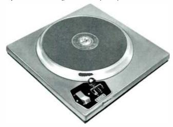
MODEL CB-77: Chassis only, ready to attach pickup arm of your choice. For 33 1/3, 45 and 78 RPM with fast pickup-to-speed and low -45 db rumble at 33 1/3 and 45 RPM. Incorporates hysterisis synchronous motor.
