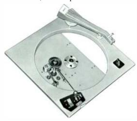
CB-510 turntable with platter removed showing the shift mechanism. The transistorized preamplifier bolts to the under side of the turntable chassis and has its own selfcontained silicon power supply.
