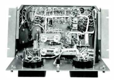
Front Panel Hinges Down for Complete Accessibility.
