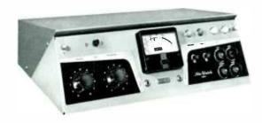
Nite-watch consists of three basic equipments supplied as a complete package: (1) production console, (2) tape control unit, and (3) the 100 record (up to 200 plays, both sides) 45 RPM automatic cueing transcription changer. Announcements are taped consecutively without intervening records. In the playback, announcements are automatically separated between record plays. Full editing sequence record selection and dubbing facilities are incorporated.
