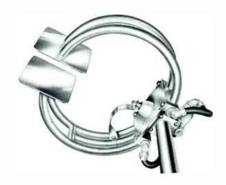
at the one megacycle bandwidth points should be expected. A side mounted antenna, pretuned at the factory should provide a voltage standing wave ratio of 1.5 to 1 or better, at one megacycle bandwidth points. The bandwidth of the Gates Cycloid antenna is ideal for stereo and multiplexing (see Figure 3) and is sufficient to minimize the detuning effect sometimes caused by atmospheric conditions.
