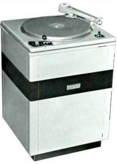
CB-525 and CB-525A turntable. This is the same as the CB-510 turntable but with the CAB-6 floor cabinet added. CAB-6 cabinet has adjustable leveling screws, full size rear door. Made of 5-ply seasoned birch, sealed and finished in gloss gray and black. Size: 21½" wide, 21½" deep, 29½" high plus 1" for leveling screws. For CB-500 chassis or CB-510 complete turntable.
