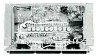
Studio unit has drop-down front panel so all parts can be reached from front of rack. Panel size of  $8\,\%$  " x  $1\,9$ " conserves much needed rack panel space.
