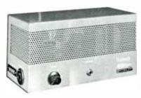
The M-5531 Unimote will perform equally well as a microphone preamplifier, turntable preamplifier, program amplifier up to 18 dbm output, repeater amplifier, isolation amplifier or as a standby amplifier for quick connection to an emergency circuit. The cover is easily removable for 100% accessibility by flipping two snap locks. Includes front panel gain control and Cannon XL-3 connector.
