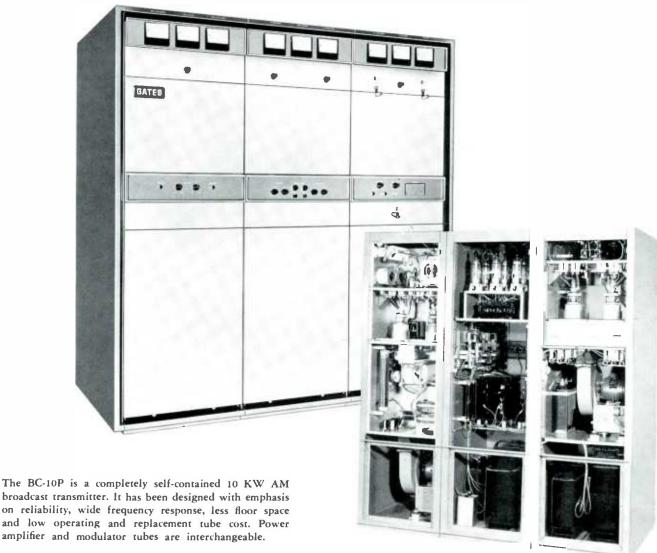
broadcast transmitter. It has been designed with emphasis on reliability, wide frequency response, less floor space and low operating and replacement tube cost. Power amplifier and modulator tubes are interchangeable.
