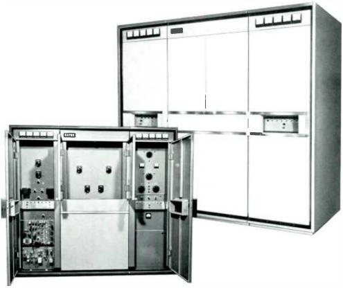
DESIGNED FOR 20 KILOWATTS — Gates engineering objective for the FM-20B was to design a completely self-contained 20-KW transmitter. The result is broadcasting's most compact 20 kilowatt FM transmitter with many inherent advantages in its design. As there is only one amplifier for 20 kilowatts output, installation is simplified and valuable floor space is saved. No diplexer is necessary, and only one 61/8" harmonic filter and one internal plate transformer is required.
