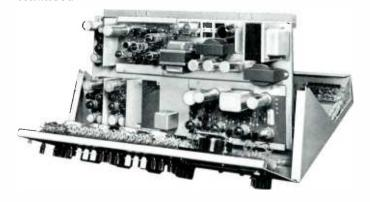
Studioette top cover is completely removed. Front panel hinges out to reach every "behind the panel" component. The amplifier deck hinges up so that muting relay contacts are at finger tip when touch-up burnishing is required.
