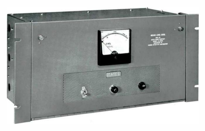
"Level Devil" accepts input signals over a 30 db range and holds the output constant (0 to +3 db). The expander threshold is -10 db relative, and below this the "Level Devil" is a linear amplifier. At this level the gain increases 10 db, and above it the amplifier acts as a peak limiter.
