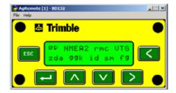
Ensure VTG is uppercase and rest are lower case. Press the  $\leftarrow$  and exit the screen. Close AgRemote return the data cable to Port A. You should now have the OmniStar set up to the right configuration and ready to work via Port A.
