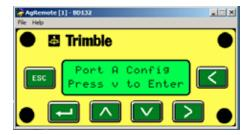
Press the v button and you will get the following screen with the correct settings. If the screen is different in any way it needs to be edited to match.
