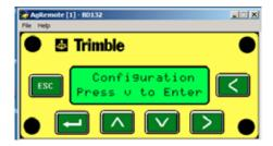
By pressing the v button first to Enter Configuration and then the < button until you get to you will get to the screen shown below which allows the configuration of Port A. (Remember you are working through Port B):
