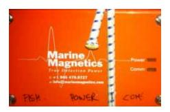
When connected to the power supply the Power LED is illuminated, when it is communicating with the fish the Comm LED flashes.
