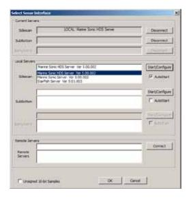
The Current Side scan Server should be LOCAL: Marine Sonic HDS and the SubBottom should be blank because we are not using one. The Local Server window AutoStart sould be selected and Marine Sonic HDS Server Ver 5.00.002 should be selected. Ignore the rest. Select Start/Configure in the Side scan and you should get the following window:
