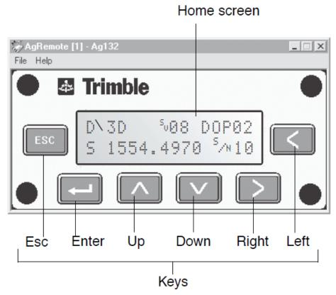
The D\3D on the Home screen means that you have differential signal. Remember, buildings can screen the OmniStar satellite so ensure that you have a clear view of the sky when doing this. The  $^s_{\nu}$  gives number of satellites. If that is OK you can close AgRemote and continue the set up of the side scan.
