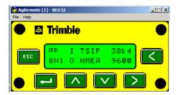
Note I means Input, that is data coming FROM the computer to the OmniLite, and usually this is irrelevant. By using the > and < buttons you can scroll around the screen to the place where you want to make a change and change, for example, what is after the I to TSIP. The communication protocol is 8N1, and finally the O = Output is NMEA and 9600. By using the  $\land$  and  $\lor$  buttons to change the setting so they match the screen above.
