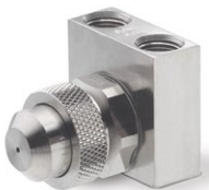
6552-1/8JAC – Miniature design is only 1/2" thick with a 1-5/32" by 1-1/4" rectangular face. The air and liquid inlets on the same side of the nozzle body – 90° to the spray direction
