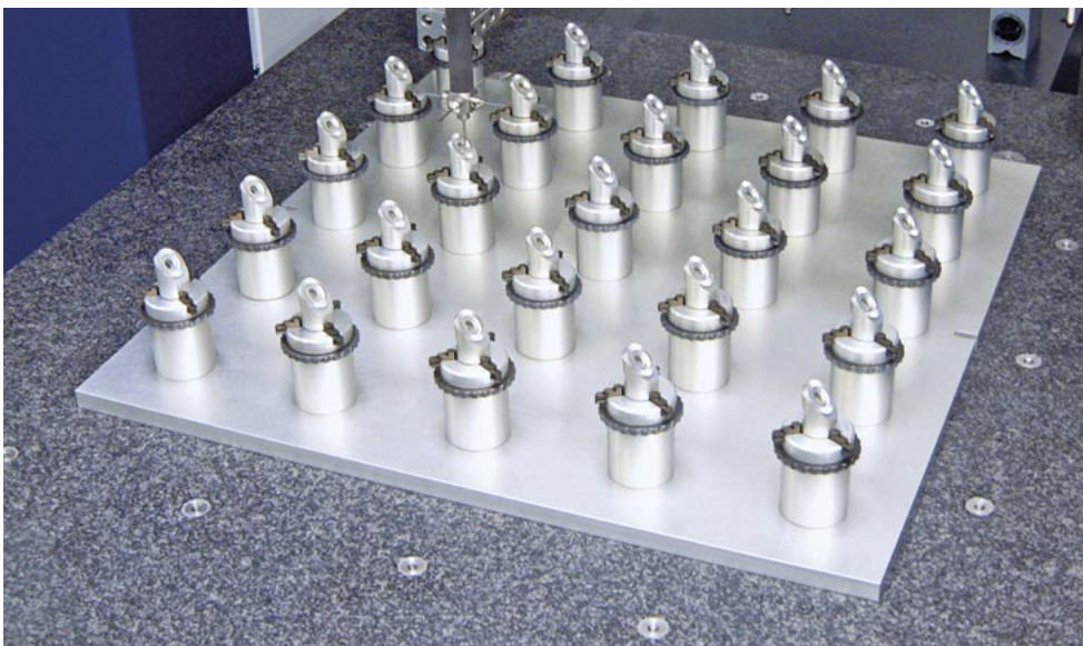
Application example 25 3-jaw keyless chucks in a measuring fixture
