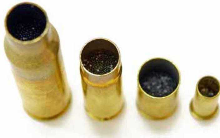
*Figure 5: Charged cases. From left to right: .308 Winchester, .300 AAC Blackout (Supersonic), 9x19mm Parabellum, .22 Long Rifle.*
