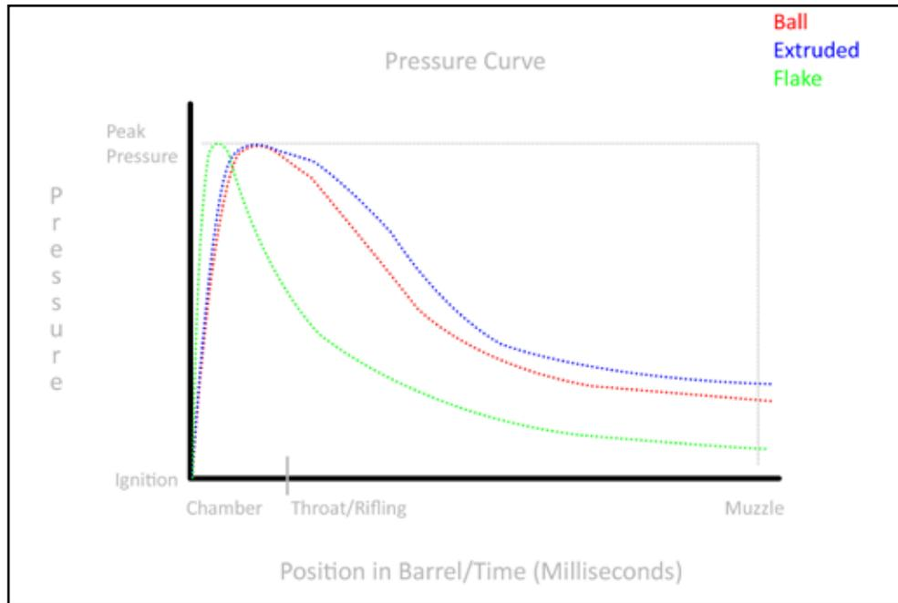
Figure 14: A comparison of propellant type pressure curves.
