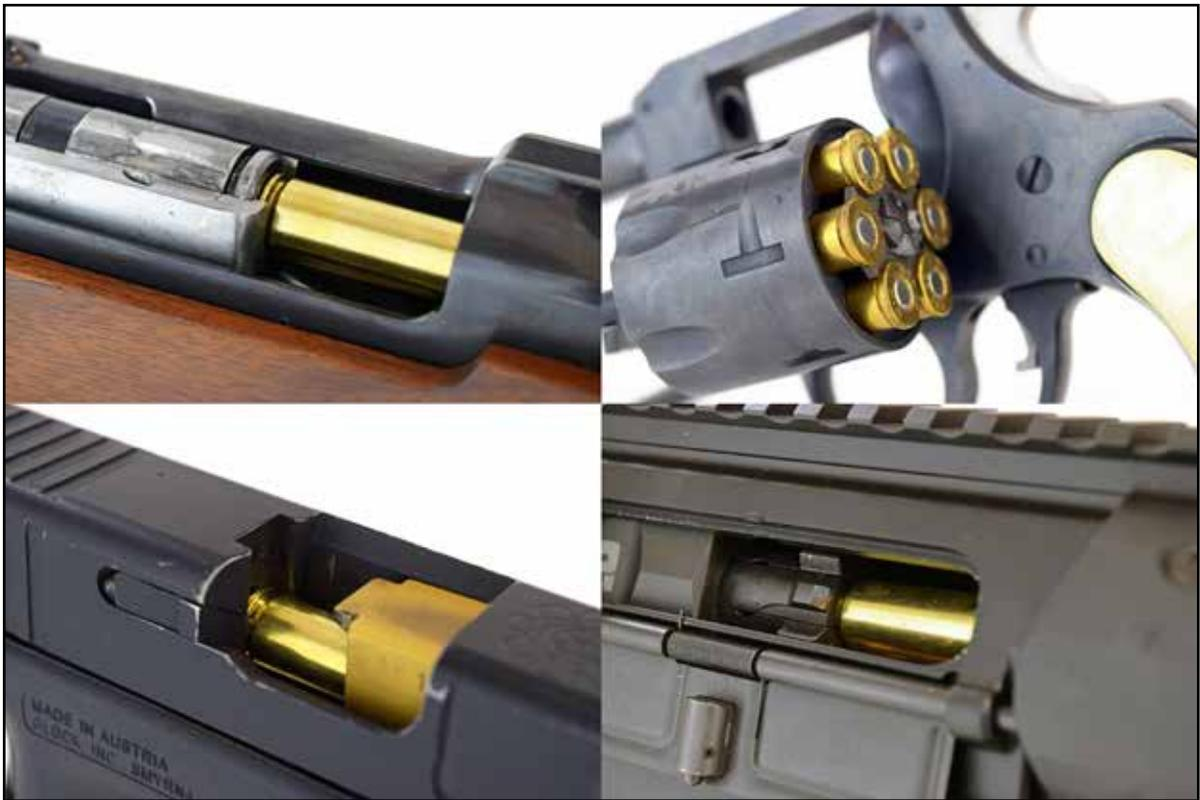
Figure 15: Various cartridges being extracted.
