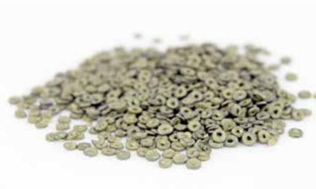
Figure 10b: Extruded tubular propellant cut into smaller disks.
