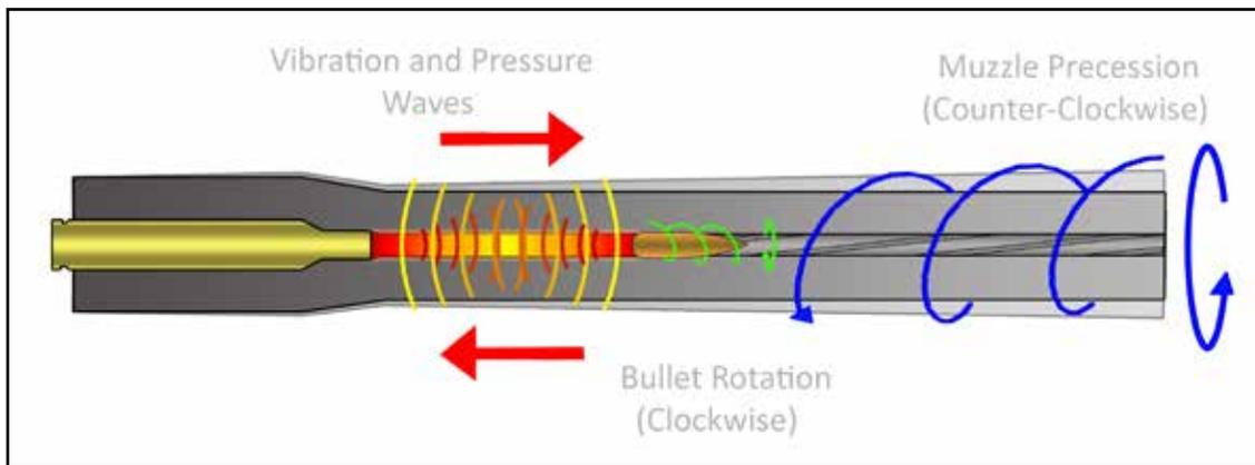
Figure 10: Barrel harmonics.
