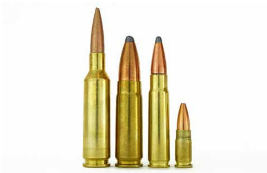
*Figure 20: Wildcat cartridges. From left to right: 6mm XC- A .250 Savage necked down to 6mm, .375 Reaper- A .308 Winchester shortened and necked up to .375, .277 Wolverine- A 5.56x45mm NATO case necked up to .277, .224 Montgomery Wildcat- A .25 ACP case necked down to .224.*
