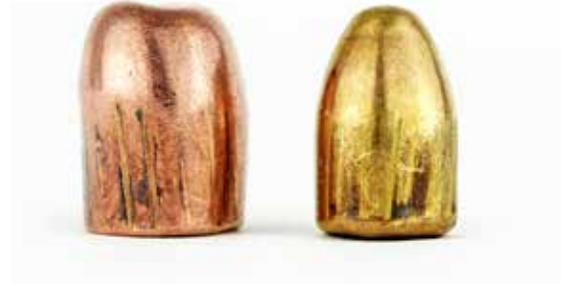
Figure 19: Recovered ball bullet from a dirt berm.
