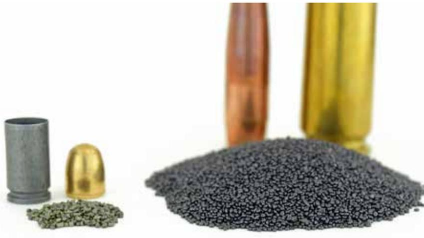
*Figure 16: A propellant charge from a .380 ACP (~3.5 grains) versus a propellant charge from a .50 BMG (~240 grains).*
