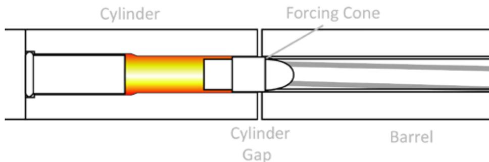
Figure 8: A .22 bullet entering the forcing cone of the barrel.
