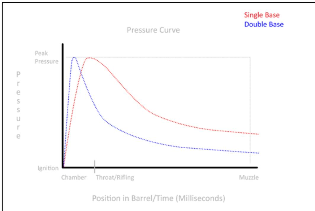
Figure 6: Single base vs. double base pressure curves.
