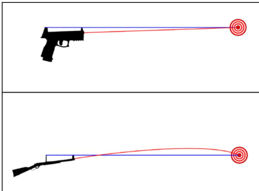
Figure 7: Single point of zero versus near/far zero.
