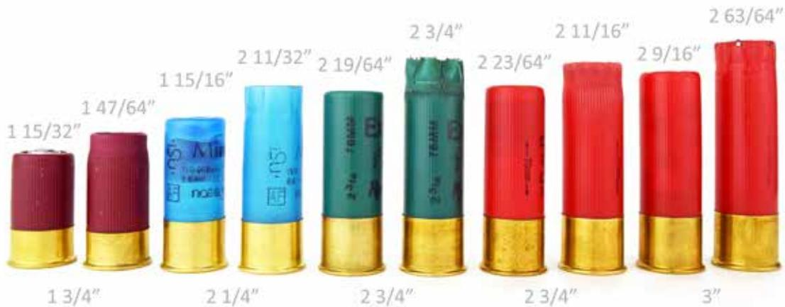
Figure 5: Shotgun shell body length before and after discharge.
