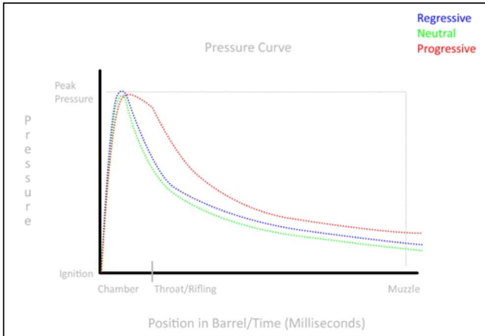
Figure 15: Burn rate pressure curves.
