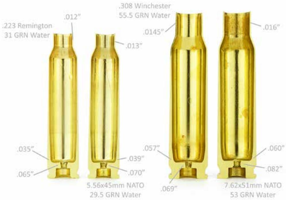
*Figure 11b: Case capacity of commercial versus military brass.*
