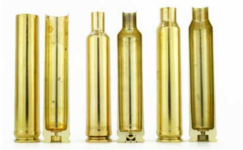
*Figure 10b: Belted case cross-sections. From left to right (pairs): .458 Winchester Magnum, .257 Weatherby Magnum, .300 Winchester Magnum.*
