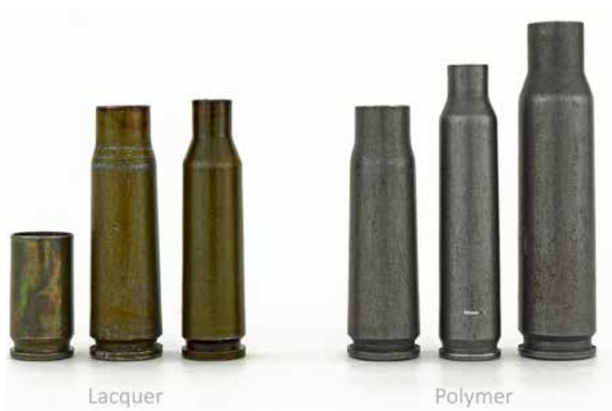
*Figure 17: Lacquer and polymer coated steel cases.*
