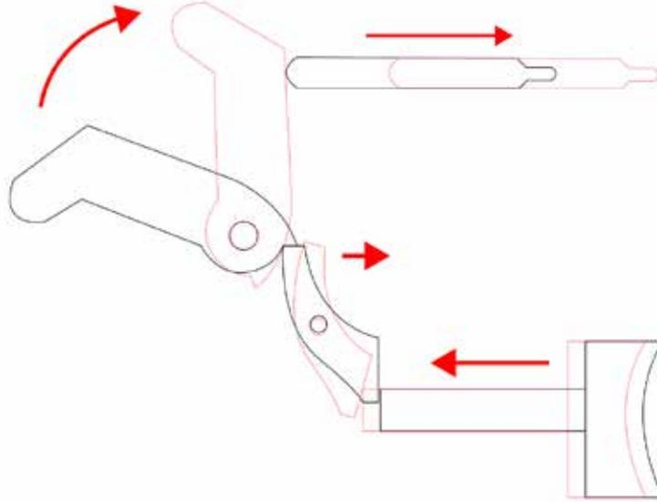
*Figure 4: Hammer-fired sequence of events.*
