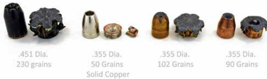
Figure 22c: Expanded hollow point bullets.
