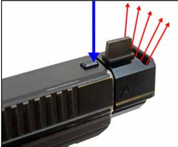
Figure 3a: How a compensator works.
