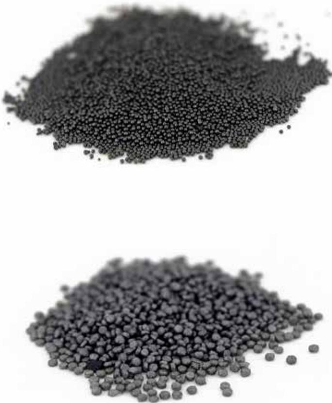
*Figure 7: Various ball and flattened ball propellants.*
