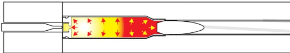
Figure 1b: As the propellant burns, the case expands and the bullet begins to move into the throat of the barrel.
