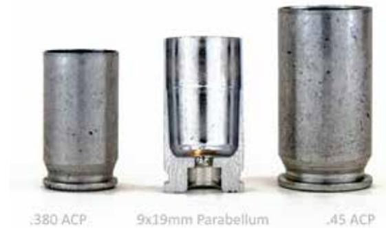
Figure 14: Aluminum cartridge cases.
