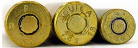
*Figure 3: Crimped primers.*
