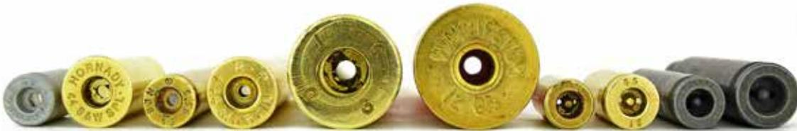
*Figure 13: Various primer pockets. From left to right: (Boxer) small pistol, large pistol, small rifle, large rifle, .50 BMG, shotshell, (Berdan) small pistol, large pistol, small rifle, large rifle.*
