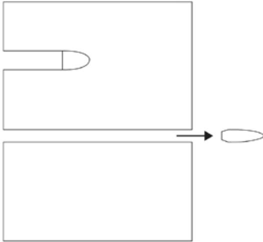
*Figure 1: Penetration vs. perforation.*
