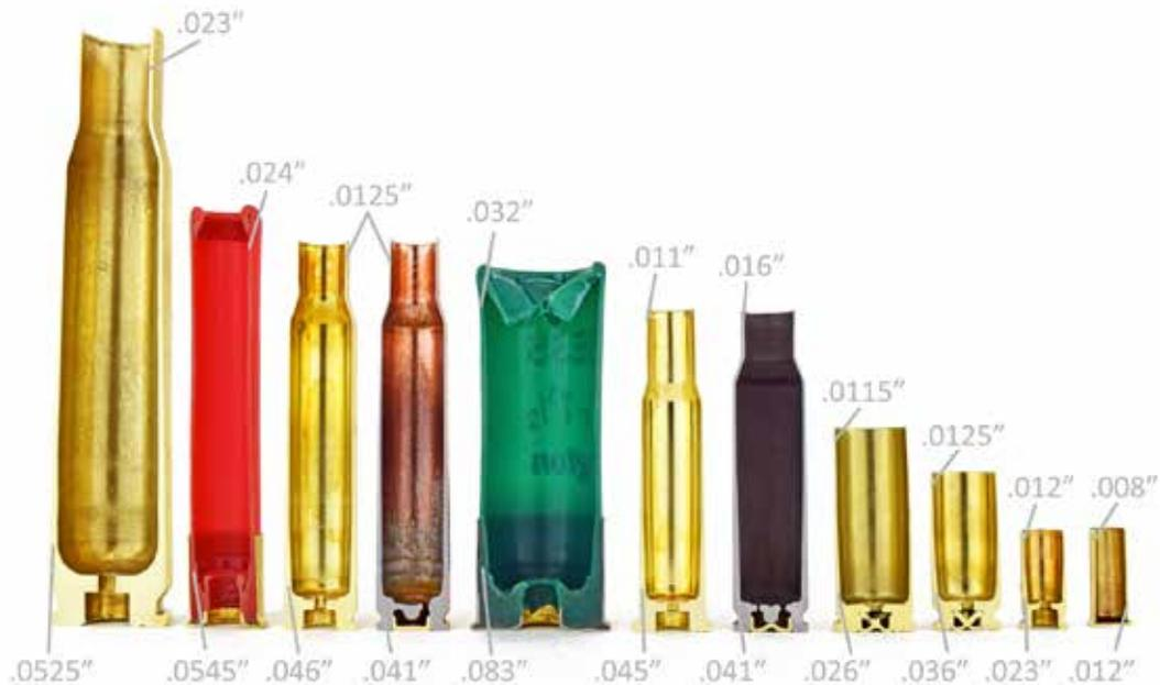
Figure 4: Various wall thicknesses. From left to right: .50 BMG, .410 Bore 3 in., .30-06 Springfield, .30-06 Springfield (steel case), 12 Gauge 2¾ in., .30-30 Winchester, .308 Winchester (steel case), .45 Long Colt, 10mm Auto, .25 ACP, .22 Long Rifle.
