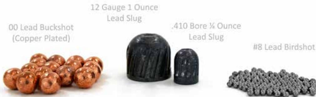
Figure 7: Various shotgun projectiles.
