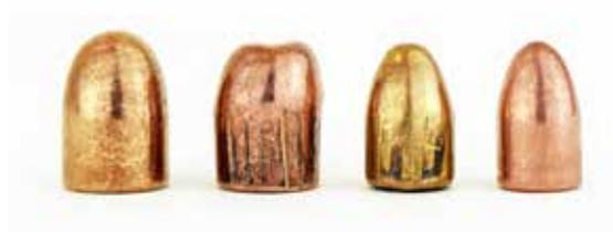
Figure 7: The body of a new bullet and the engraving of a bullet that was fired.
