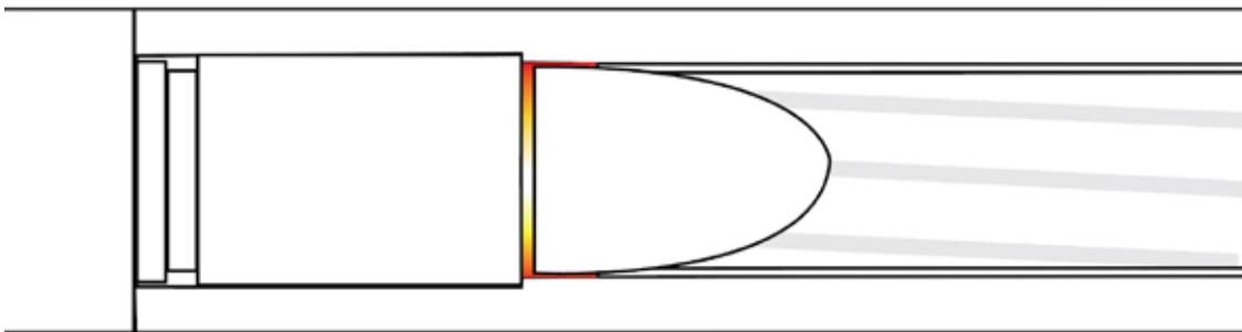
*Figure 6: 9mm bullet entering the rifling.*
