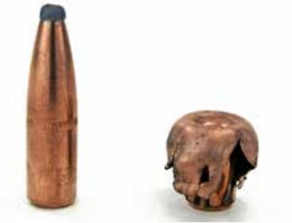
Figure 23c: Expanded soft point bullet.
