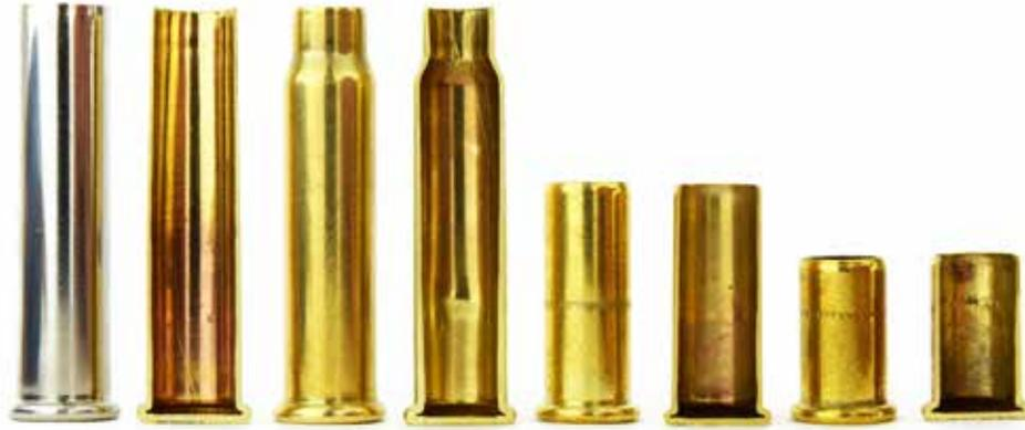
Figure 17: Rimfire cartridge rims. From left to right (pairs): .22 Winchester Magnum Rimfire, .17 Hornady Magnum Rimfire, .22 Long Rifle, .22 Short.
