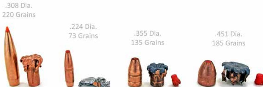
Figure 16c: Expanded polymer tipped bullets.
