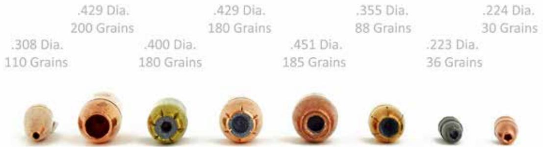
Figure 22a: Several different hollow point bullets.
