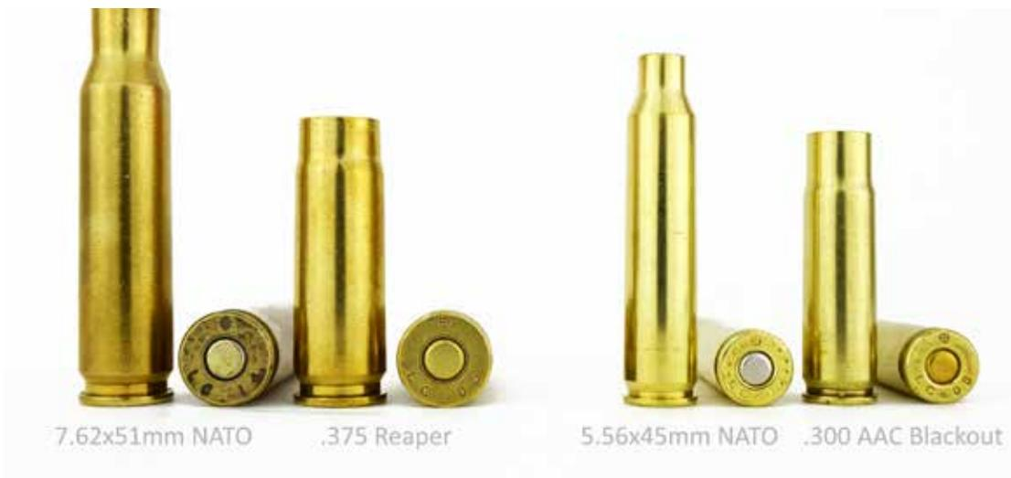
Figure 21: Modified cases. The .375 Reaper case is made by shortening and “necking” up the 7.62x51mm NATO case. The .300 AAC Blackout case is a shortened and necked up 5.56x45mm NATO case.
