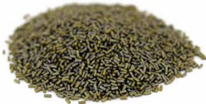
*Figure 4: IMR propellant.*
