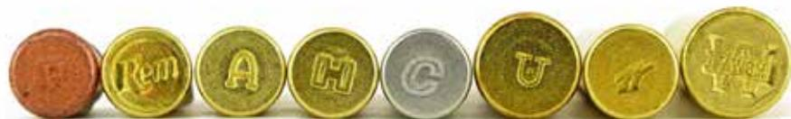
Figure 20c: Rimfire headstamps. From left to right: Henry-Winchester (H) .22 BB Cap, Remington (Rem) .22 Short, Aguila (A) .17 PMC Aguila, Hornady (H) .17 Hornady Mach II, CCI (C) .22 Long Rifle Stinger, Remington Arms Co./Union Metallic Cartridge Company (U) 5mm Remington Magnum, Winchester (W) .17 Hornady Magnum Rimfire, Winchester (W) .17 Winchester Super Magnum.
