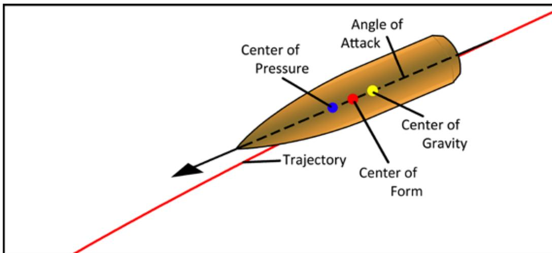
Figure 4: The projectile's center of form, gravity, and pressure.
