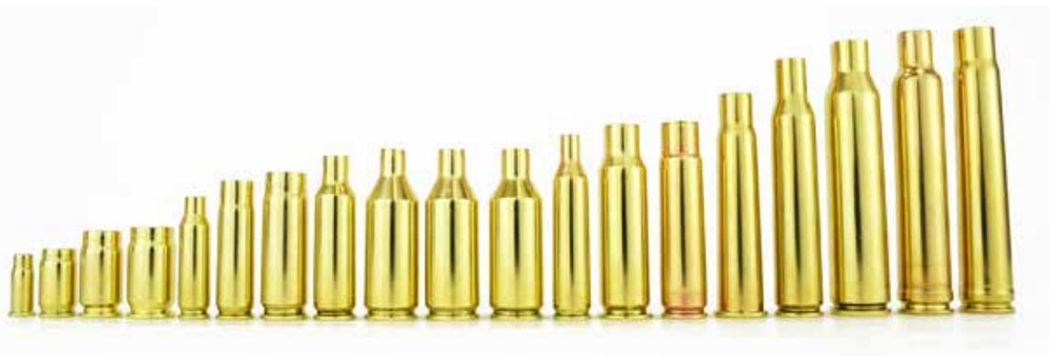
Figure 9a: Bottleneck cases. From left to right: .17 PMC Aguila, .32 NAA, .357 SIG, .400 Corbon, HK 4.6x30mm, .300 AAC Blackout, .375 Reaper, .224 Valkyrie, .223 Winchester Super Short Magnum (WSSM), .243 WSSM, .25 WSSM, .17 Remington, .338 Marlin Express, .35 Remington, .303 British, .270 Winchester, .338 Lapua Magnum, .300 Weatherby Magnum, .375 H&H Magnum.
