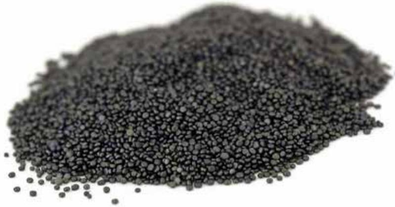
*Figure 5: Ball propellant.*
