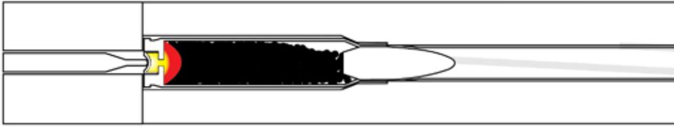
Figure 1a: The firing pin crushes the primer and initiates ignition.
