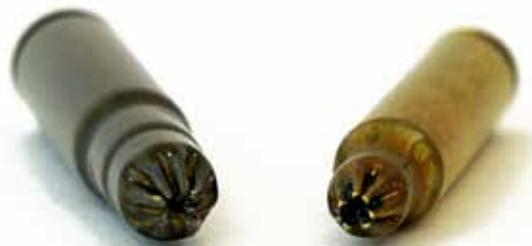
*Figure 12: Blank cartridges with star crimps.*
