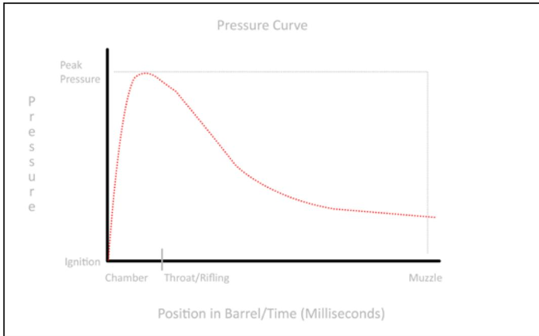
Figure 8: Ball propellant pressure curve.
