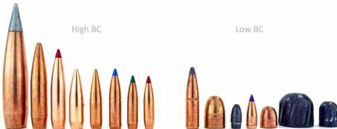
Figure 40: Various projectile BCs. All BCs in G1.
