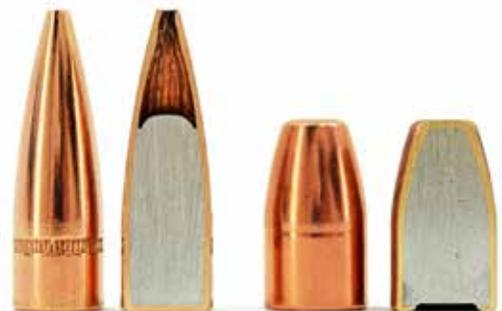
Figure 28: Zinc core rifle and pistol bullets.
