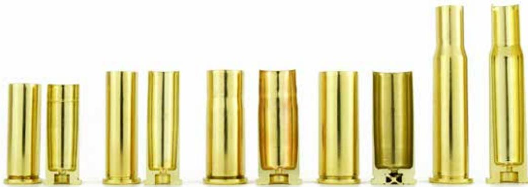
Figure 3b: Rimmed case cross-sections. From left to right (pairs): .38 Smith & Wesson Special, .357 Smith & Wesson Magnum, .44-40 Winchester, .45 Colt, .30-30 Winchester.
