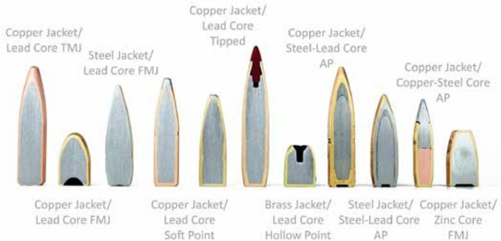
Figure 5: Various bullet cores.
