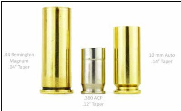
Figure 7a: Straight-walled cases with a slight taper.
