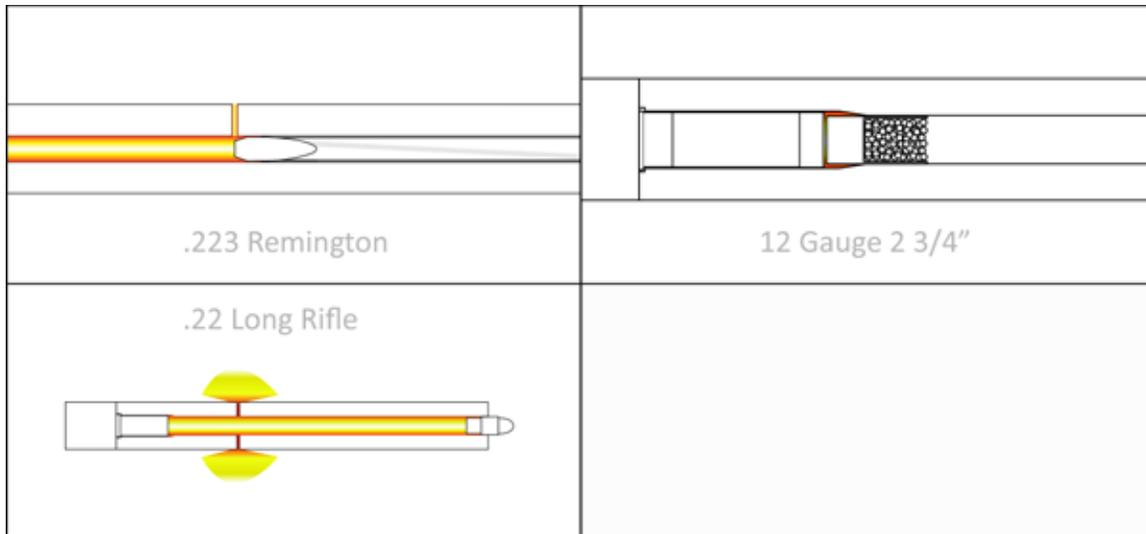
Figure 12: Projectile position at .5 milliseconds.
