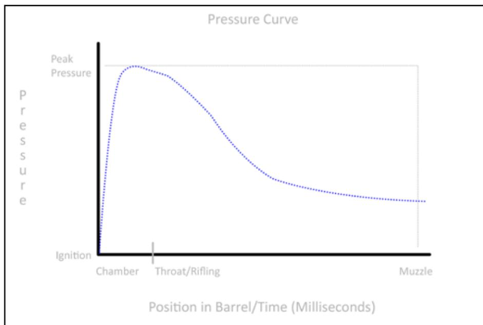
Figure 11: Extruded propellant pressure curve.
