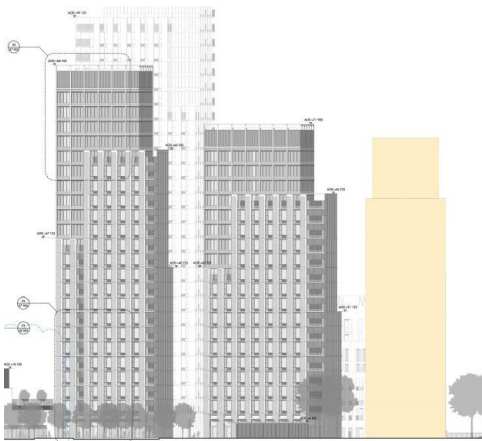
Image 09 (above): Early iteration of the scheme proposing a 20 storey tower (depicted in yellow).
