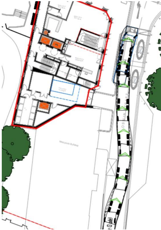
Image 39 (above): Tracking diagram of a refuse vehicle negotiating the cycle shelter on Oswin Street.
