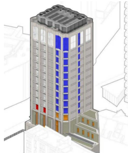
Image 22 (above): Isometric of the building, showing the proposed treatment to the south and west facing glazing
