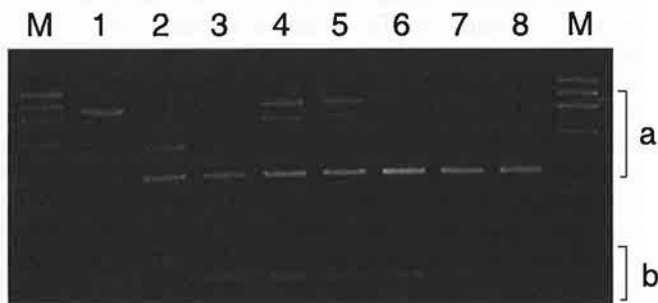
Fig. 2. PCR amplification of genomic DNA of two maize inbred lines Ac7643S5 and CML247, and 6 F2 plants from the cross of these two lines with two primer sets (for umc67 sts and MAG1A01) in the same PCR reaction. M, HaeIII-phiX174 size marker. The amplification products were fractionated in 3% MetaPhor agarose gel in 1X TBE buffer.
