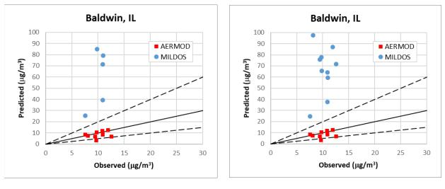
(a) Momentum plume rise (receptors R2 – R5 and R10 are off-scale) (b) Buoyant plume rise
