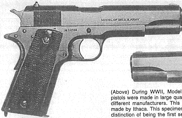
(Left) The 1911 Colt, a single-action pistol, is considered by many to be the best semi-automatic pistol ever designed. It was adopted by the U.S. Army in 1911 and is still in limited military service.
