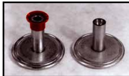
Wedge Piston Assembly Meritor Bendix
