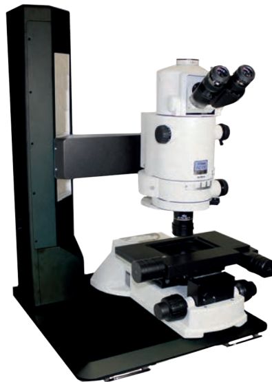
Nikon AZ100 mounted on a ProZ stand, with a Prior motorized stage and a Nikon AZ-STD base.
