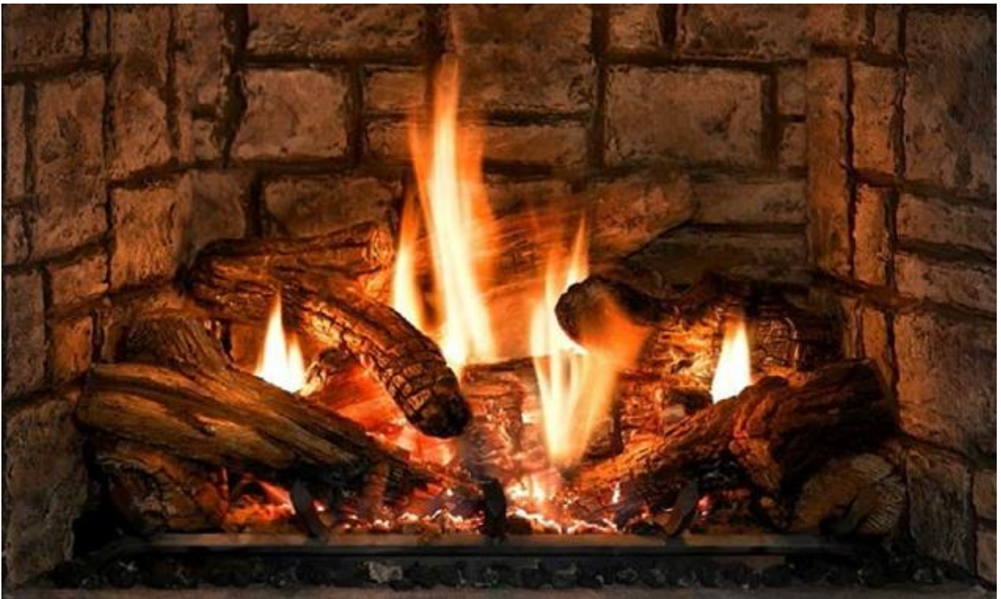
Figure 6-1 Burner Flame Heights: This image provides a visual reference for the burner flames burning at maximum height after the burners have been operating for 30 minutes or longer. A normal rear flame will be 1 to 2 inches above the rear log top edge. This, however, is dependent on the gas type, air shutter opening setting and vent system configuration. Actual flame heights can be slightly higher or lower when compared to this reference image.
