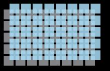
**Pixel Scaling** 4K Enhancement Technology<sup>2</sup> shifts each pixel to double HD resolution on-screen.
