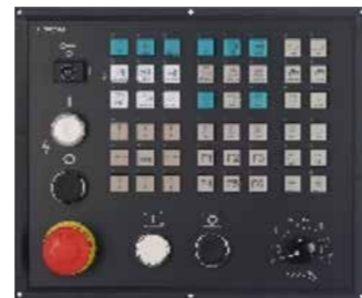
Control Panel for Mill
