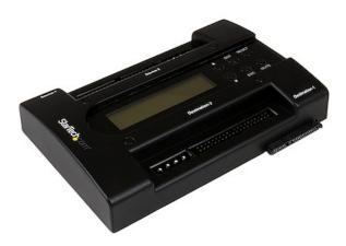
The UNIDUPDOCK Universal SATA/IDE Dual Hard Drive Duplicator functions as both a convenient solid state (SSD) or hard drive (HDD) copying/imaging solution or an external SATA/IDE SSD or HDD docking station for 2.5in or 3.5in drives (SATA, SATA II, SATA III).
