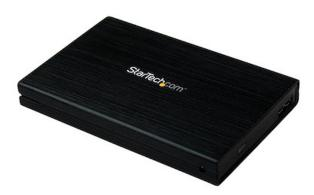
The S2510BMU33 USB 3.0 Hard Drive Enclosure with UASP lets you connect a 2.5in SATA III hard drive (HDD) or solid state drive (SSD) through an available USB port. The enclosure delivers optimal performance with a USB 3.0 connection, but is backward compatible with USB 2.0/1.1 host connections as well.
