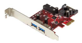
This PCI Express USB 3.2 Gen 1 card offers a cost-effective upgrade that lets you add four USB 3.2 Gen 1 ports to your computer through a PCIe slot. It offers two external ports plus two internal (IDC) USB 3.2 Gen 1 headers to help adapt your desktop or server to support a variety of USB 3.2 Gen 1 devices.
