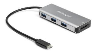
Expand the connectivity of your USB-C laptop with this bus-powered 3-Port USB-C hub. It plugs into your laptop's USB Type-C or Thunderbolt 3 port, adding three USB-A ports and an SD card reader, so you can quickly connect more peripherals and devices.
