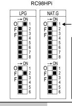
Move switch 1 to OFF for long flue lengths. See below.
