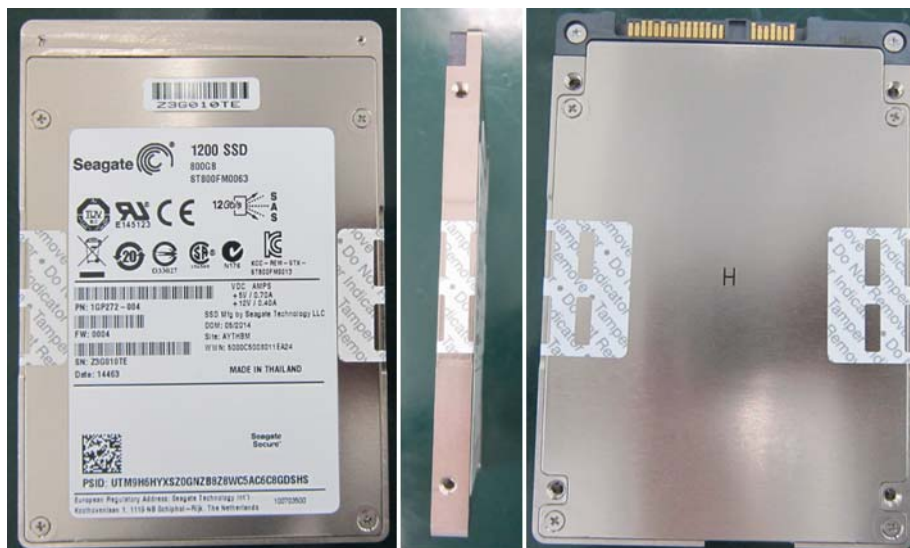
Figure 7 Example of FIPS tamper evidence labels
