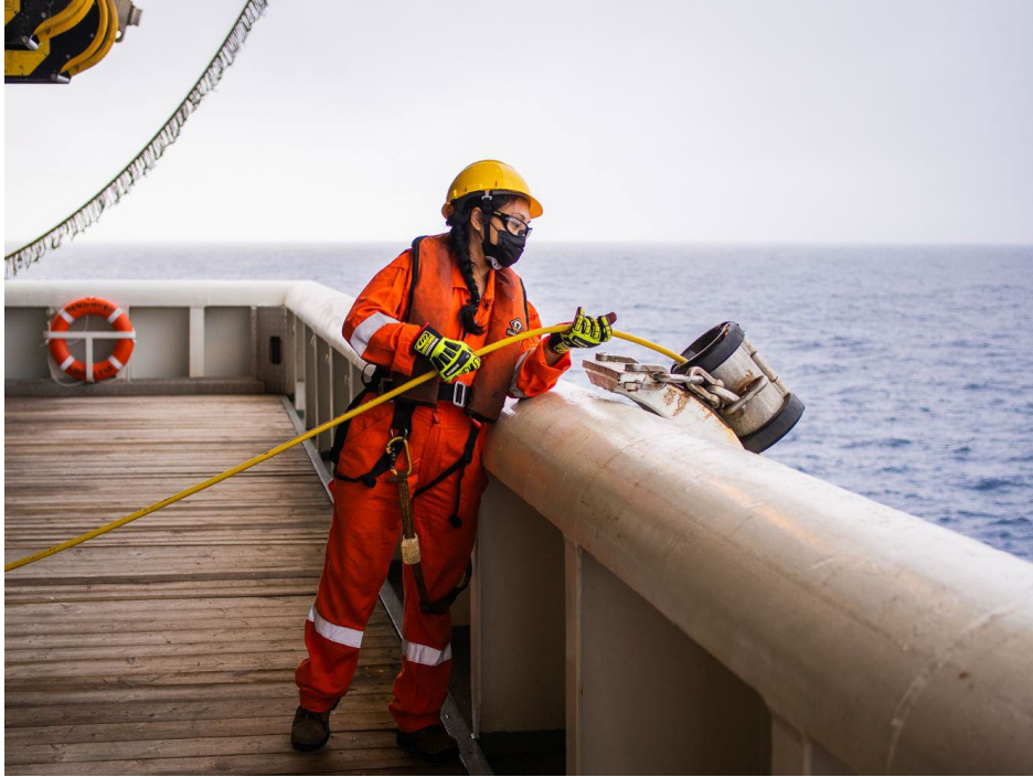
Figure 3. PAM operator manually feeding tow cable through sliding collar on stern
