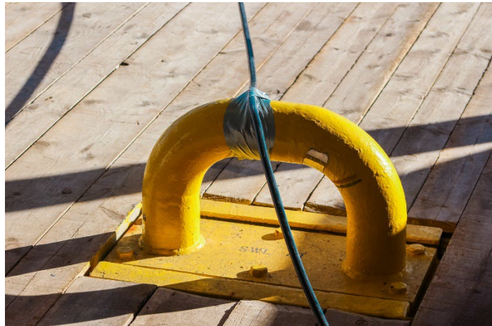
Figure 10 . PAM cable marked at winch; excess cable taped on streamer deck
