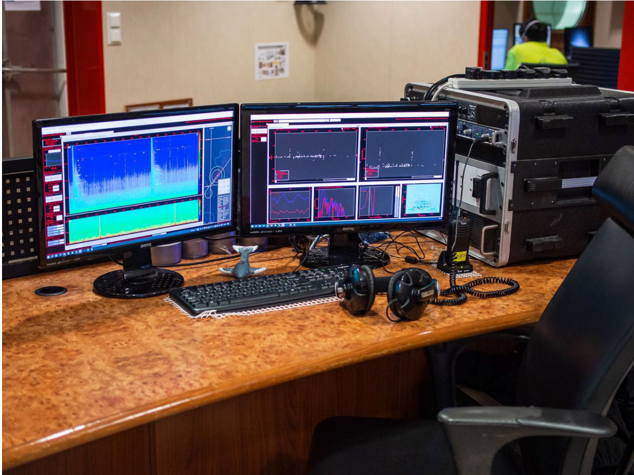
Figure 11: Passive acoustic monitoring station in instrument room.
