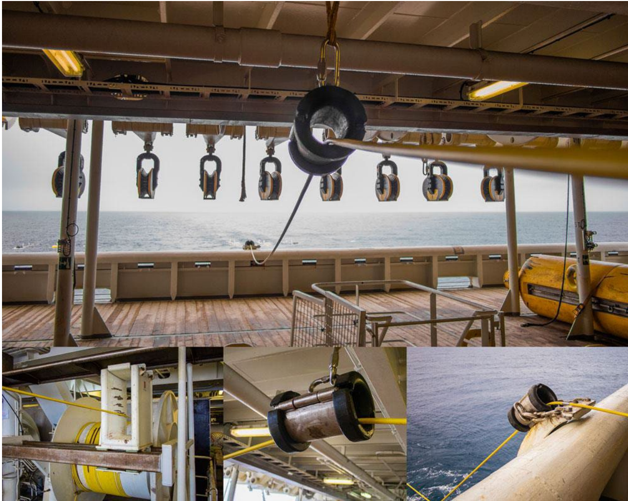
Figure 2. Deployed of tow cable showing directionality, position on winch, sliding collar from ceiling, and sliding collar at the ships stern.
