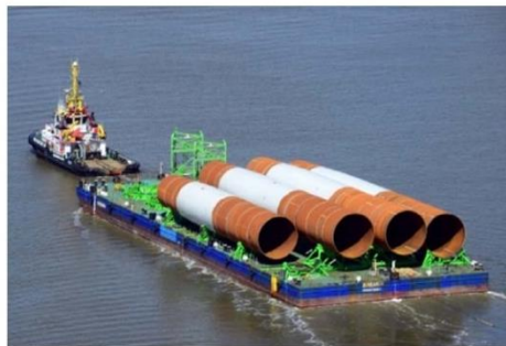
Monopile Transport via Tugboat and Barge
