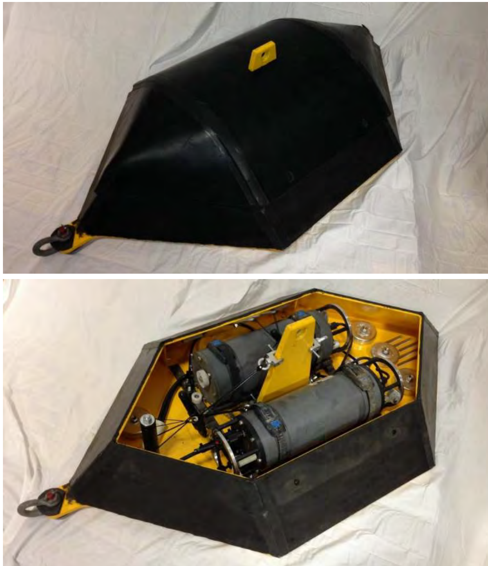
Figure 3. Photos of mooring for proposed sound level measurements of DTH hammering. Top: high-flow mooring. Bottom: high-flow mooring with cover removed to show two AMAR recorders within the mooring.
