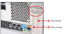
2. Install the PCle x4 / PCle x16 card into the PCle x4 / PCle x16 slots
