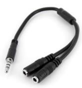
The MUYHSMFF Headphone/Microphone Combo Jack splitter (4-position 3.5mm to dual 3-position 3.5mm) is a headset Splitter Adapter that features one 3.5mm Male (TRRS) and two 3.5mm (TRS) Female connectors, enabling you to add a mono microphone input, as well as a stereo output to your PC or Laptop, through a single 3.5mm audio port.
