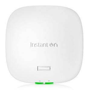
The HPE Networking Instant On Access Points AP32 is a Wi-Fi CERTIFIED™ 6E access point that brings a 6Ghz dedicated band to support Wi-Fi 6 capable devices. With this dedicated band you'll experience lower latency and faster transmit rates (up to 3.6 Gbps) for your Wi-Fi 6 enabled devices. Support over 100 devices with this 2x2 tri-band wireless access point and bring the cloud closer to your edge.
