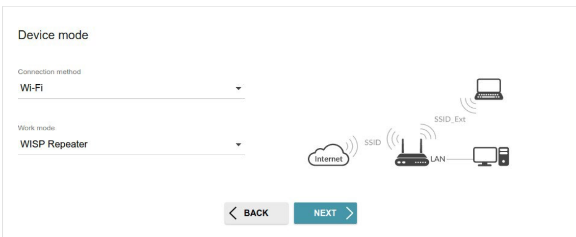
Figure 37. Selecting an operation mode. The WISP Repeater mode.
