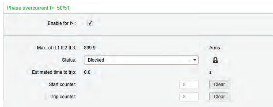
Figure 41 - Result for the I> stage when the DI is active and the stage exceeds its current start value
