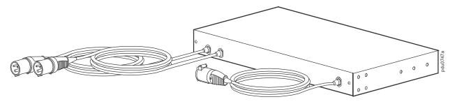
**Input power cords:** The two IEC 309-16 A, 3-pin plug cords connect the switch to two separate power sources (A, B). The switch is set to draw power from the preferred source and to automatically switch over to the secondary source when necessary.
