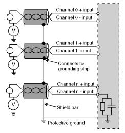
If the sensors are referenced in relation to the ground, this can return a remote ground potential to the terminal block. To help avoid this situation, follow these rules:
