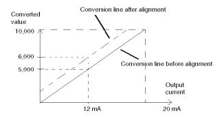
The alignment value is editable from a programming console, even if the program is in RUN mode. For each output channel, you can:
