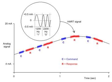
These digital signal frequencies are higher than the typical analog signaling frequency range of 0...10 Hz. The digital signal is typically isolated using a passive high-pass filter with a cut-off frequency in the range of 400...800 Hz. The analog signal is likewise isolated using a passive low-pass filter.
