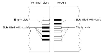
The diagram below shows an example of a coding configuration that makes it possible to fit the terminal block to the module.
