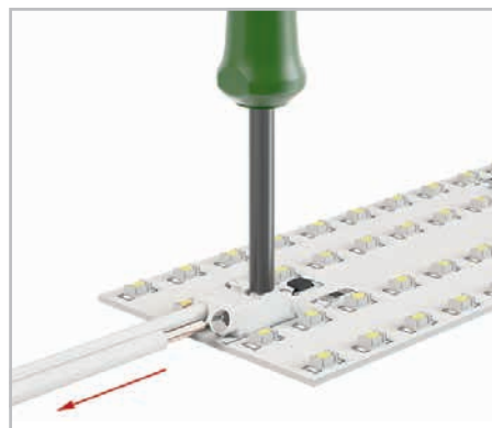
Inserting/removing fine-stranded conductors by lightly pressing on push-button (e.g., using a 206-861 operating tool).
