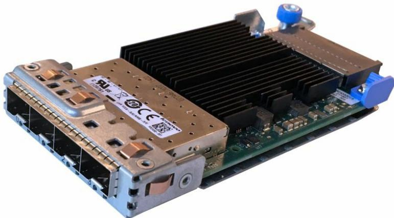
Figure 4. ThinkServer X710-DA4 AnyFabric 10Gb 4 port Ethernet Adapter by Intel
