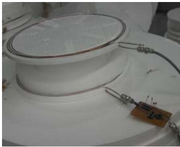
Figure 7b: transmitting antenna with tuning circuit and receiving antenna used in experiments.
