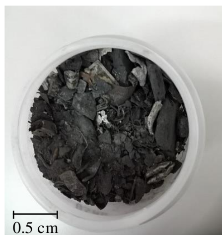
Figure 3. Solid WPCBs material after thermal pre-treatment and the I leaching ( 4M H_2SO_4 + 100 g/dm^3 (NH_2)_2CS + 13 g/dm^3 Fe_2(SO_4)_3 ).
