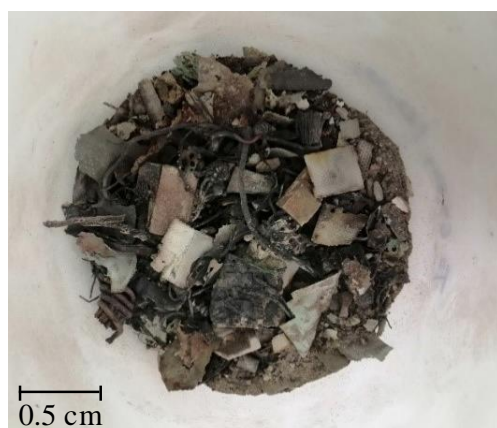
Figure 2. Solid WPCBs material after thermal pre-treatment at the temperature T = 1023 K for 7 h.
