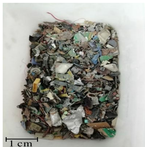
Figure 1. Solid WPCBs starting material.
