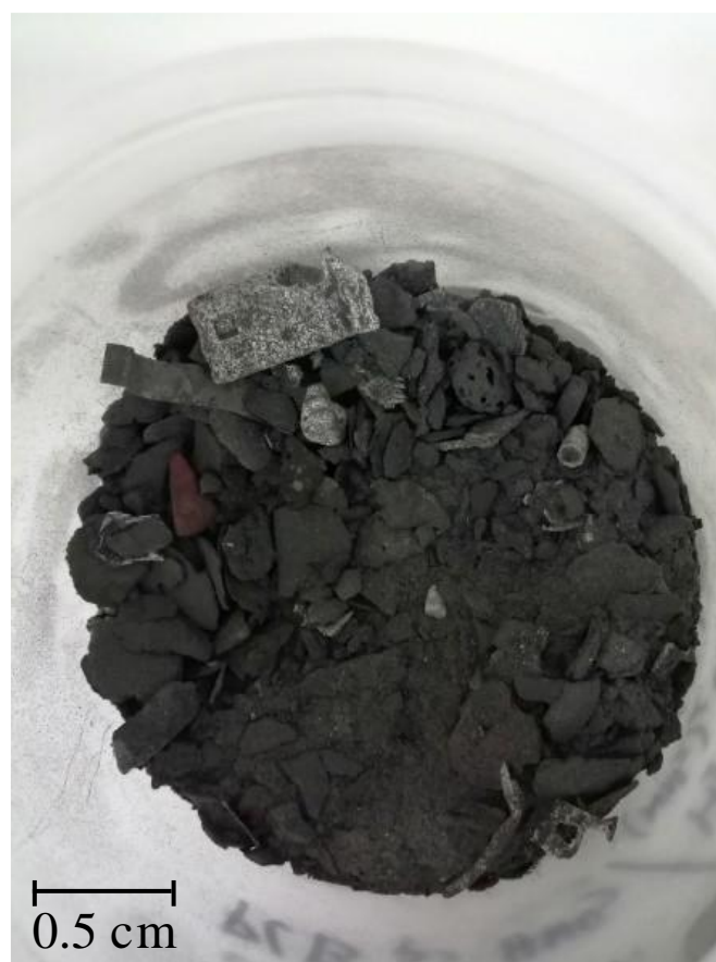
Figure 4. Solid WPCBs material after thermal pre-treatment and two steps of the II leaching with 5M HNO 3 and (4M H 2 SO 4 + 100 g/dm 3 (NH 2 ) 2 CS + 13 g/dm 3 Fe 2 (SO 4 ) 3 ), respectively.
