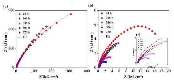
**Figure 8.** EIS Nyquist diagrams with a respective fitting line for SS 430 and carbon steel B450C after different times of immersion in chloride-containing (5 g  $L^{-1}$  NaCl) cement extract solution: (**a**) SS 430, (**b**) B450C and (**c**) zoom of B450C (**b**) diagram.
