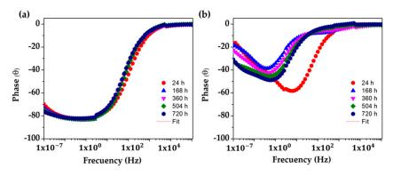
**Figure 10.** EIS Bode diagrams with a phase angle with a respective fitting line for SS 430 and carbon steel B450C after different times of immersion in cement extract solution (+5 g  $L^{-1}$  NaCl): (a) SS 430, (b) B450C.
