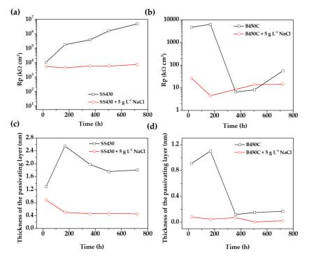
**Figure 12.** (**a**,**b**) Evolution of  $R_p$  values and (**c**,**d**) passive layer thickness (*d*) during the immersion of SS 430 and carbon steel B450 to cement extract solution in the presence of chloride-containing cement extract solution (this study) and in the absence of chlorides [34].
