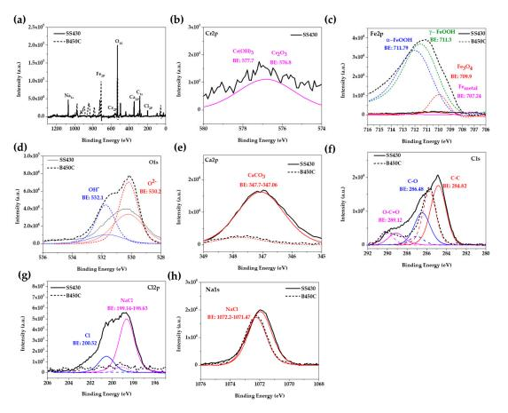
**Figure 6.** Overview of X-ray photoelectron spectroscopy (XPS) spectra acquired from SS 430 and carbon steel B450C after exposure to cement extract solution (+5 g L<sup>-1</sup> NaCl) for 30 days: (**a**) full spectrum; spectrum for (**b**) Cr2p; (**c**) Fe2p; (**d**) O1s; (**e**) Ca2p; (**f**) C1s; (**g**) Cl2p and (**h**) Na1s.
