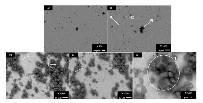
observed (compared to that of carbon steel B450C, Figure 2) and only selected areas were covered, mainly by crystals of CaCO<sub>3</sub> and NaCl (Table 6).
