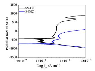
**Figure 7.** Potentiodynamic polarization curves of SS 430 stainless steel and B450C carbon steel exposed to the cement extract solution (+5.0 g  $L^{-1}$  NaCl).
