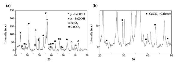
**Figure 3.** XRD spectra of corrosion products formed on B450C carbon steel surface (**a**) and CaCO<sub>3</sub> spectra (**b**) after 30 days of exposure to chloride-containing cement extract solution.
