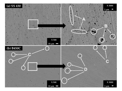
**Figure 1.** SEM images (×500) of surface steel control samples and zoom (×3000) of areas of interest: (**a**) SS 430 and (**b**) carbon steel B450C.
