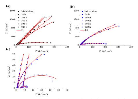
**Figure 9.** EIS Nyquist diagrams with a respective fitting line for SS 430 and carbon steel B450C after different times of immersion in cement extract solution: (a) SS 430, (b) B450C and (c) zoom of B450C (b) diagram [34].
