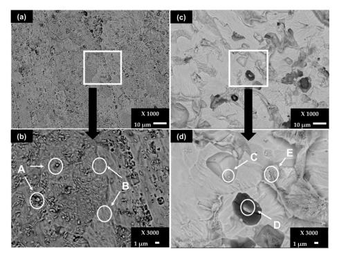
**Figure 5.** SEM images ( $\times$ 1000) of steel surfaces after removal of corrosion layers formed during exposure to chloride-containing cement extract solution for 720 h (30 days): (**a**) SS 430 and (**b**) zoom ( $\times$ 3000); (**c**) B450C and (**d**) zoom ( $\times$ 3000).
