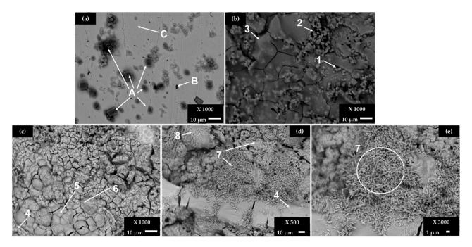
**Figure 2.** SEM images of B450C carbon steel exposed to a cement extract solution (+5 g L<sup>-1</sup> NaCl): (a) a less corroded area and (b) a more corroded area after 168 h (7 days); (c–e) after 720 h (30 days).
