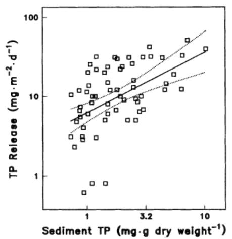
FIG. 3. Regression of TP release rates on sediment TP concentration after logarithmic transformation with literature data on lakes worldwide. The regression line and 95% confidence band are shown (log RR =  $0.80 + 0.76 \log \text{TP}$ ,  $r^2 = 0.21$ , n = 63).
