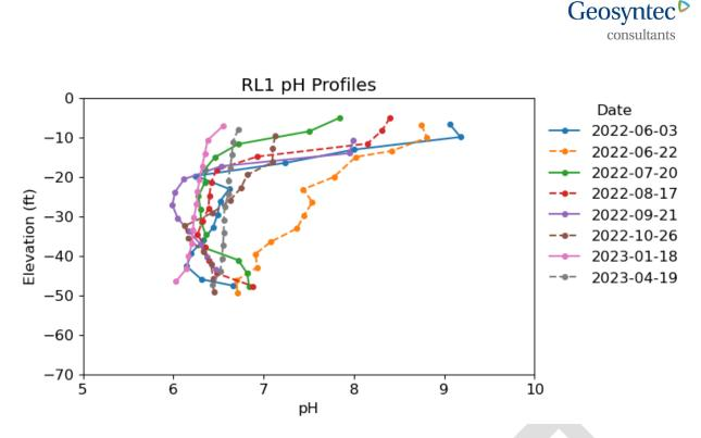
Figure 19. Vertical pH profiles at RL1
