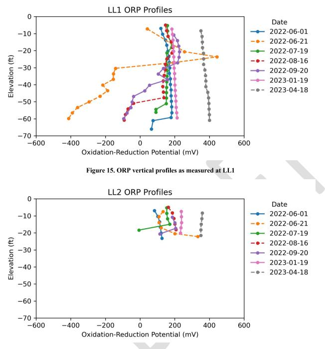
Figure 16. ORP vertical profiles as measured at LL2
