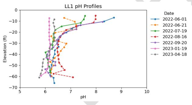
Figure 11. pH vertical profiles as measured at LL1
