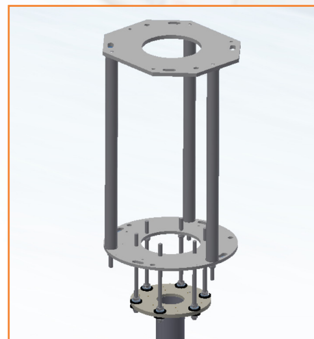
Substructure with Adaptor Plate (H2P01) and Extension to bridge large gaps
