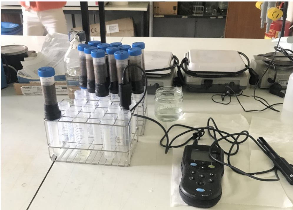
Figure 2.5: Maintenance of the columns with the multimeter.
