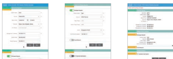
3-step over-the-air wireless network configuration
