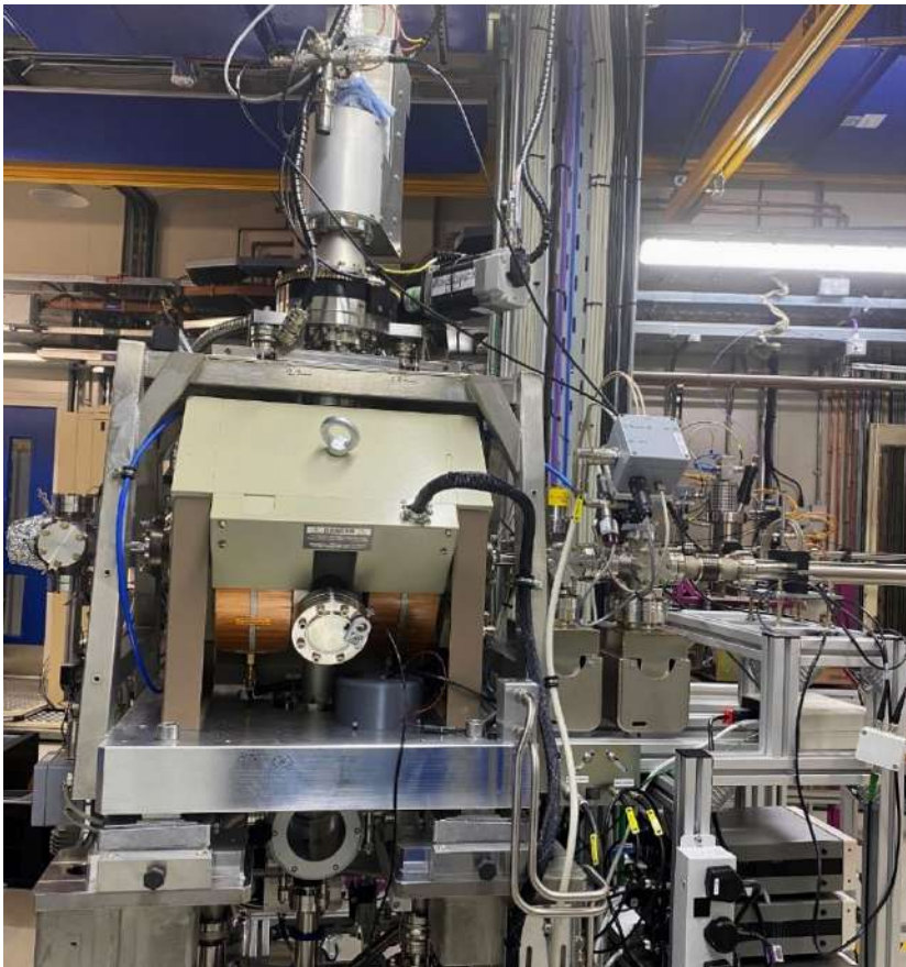
Figure: Image of the electromagnet end-station connected at the end of the absorption branch of I10.
