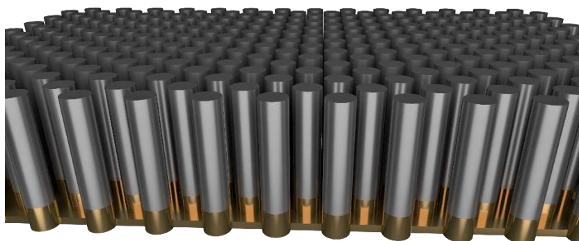
Figure: Nanowire arrays prepared by electrochemical deposition
