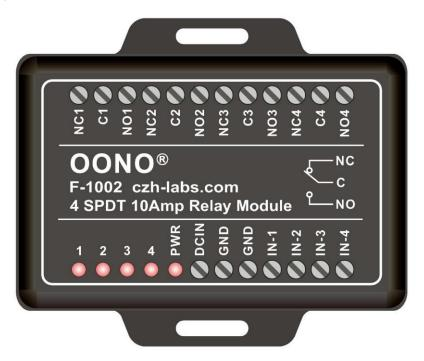
DC IN: Operating power supply input (V+).
