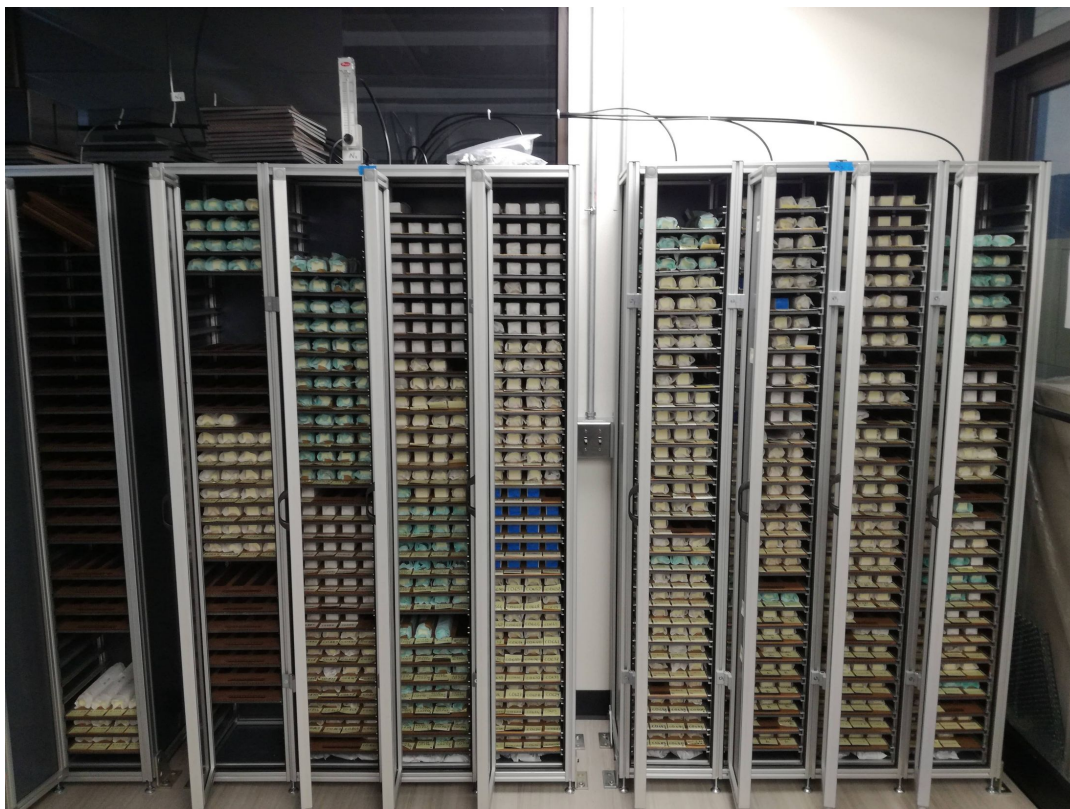
Figure 5.1: CsI crystals which have been tested for geometry and optical properties. They are placed into nitrogen fluxed cabinet waiting to be installed inside the calorimeter disk.
