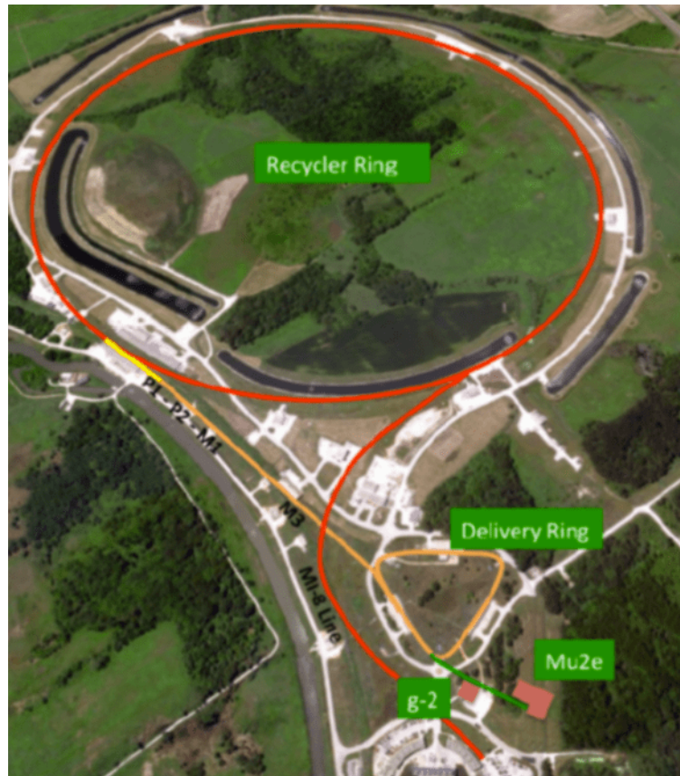
Figure 1.3: Layout of the Mu2e facility (lower right) relative to the accelerator complex that provides the proton beam to the detector. Protons are transported from the Booster through the MI-8 beamline to the Recycler Ring, where they circulate while being rebounded by a 2.5 MHz RF system. The reformatted bunches are kicked into the P1 line and transported to the Delivery Ring, where they are slowly extracted for the Mu2e detectors
