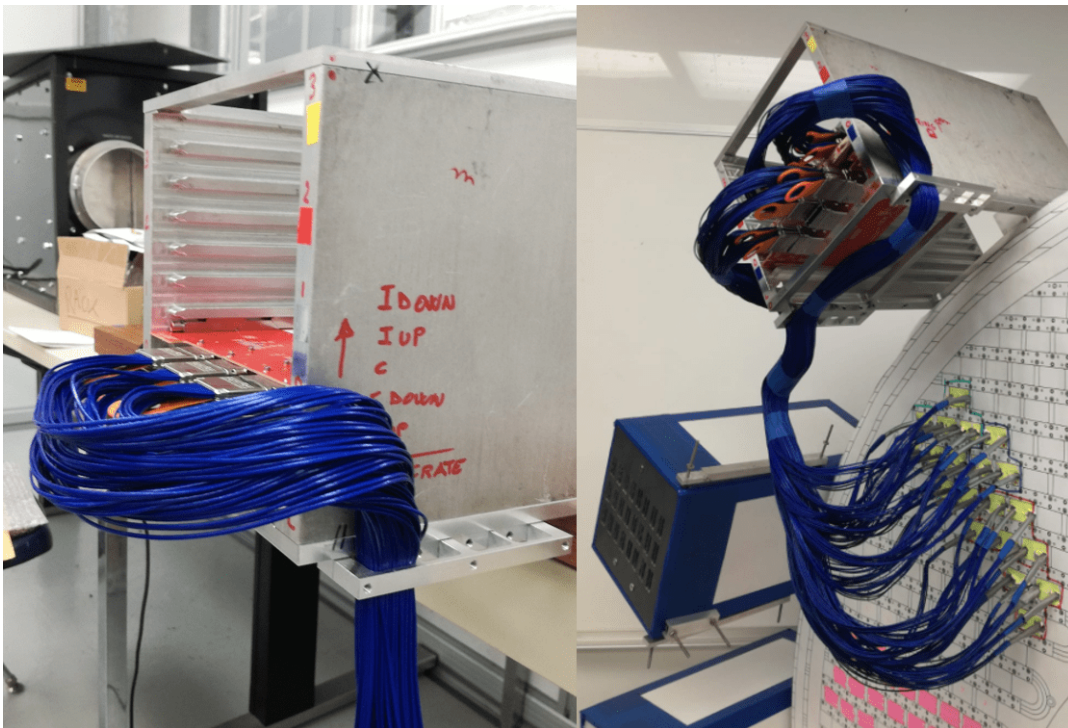
Figure 23: The FEE cable set-up to shape cables in the final form
