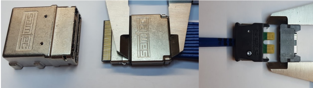
Figure 17: The FEE cable connectors: the HDLSP at left and the ECDP-04-L2 at right.
