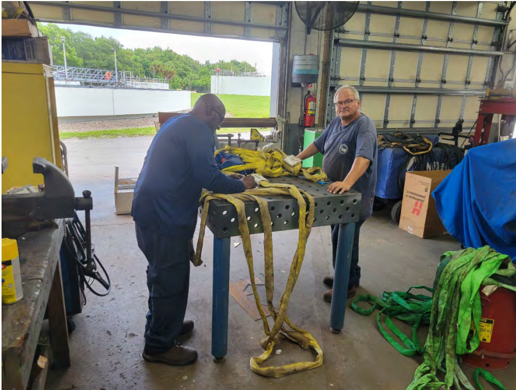
Maintenance Team Members Performing Safety Inspection of Lifting Straps
