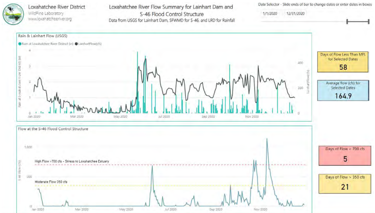
Flow measurements for 2020 through the Lainhart Dam superimposed with daily rainfall measured at the LRD plant site (top) and the S-46 control structure (bottom).
