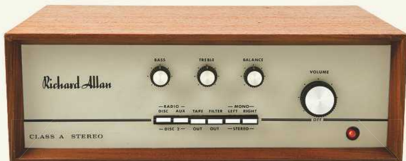
ABOVE: The Richard Allan A21 was the first Class A transistorised amp on the UK market
