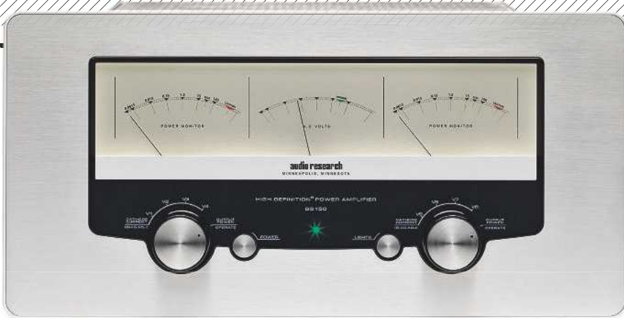
ABOVE: Dominating but also graceful, ARC's trio of analogue meters conveys a measure of mains line voltage, tube bias current (in adjustment mode) and power output. The log scaling of the latter seems of decorative value only as a sustained 10W/8ohm registered just '0.015' on the display
