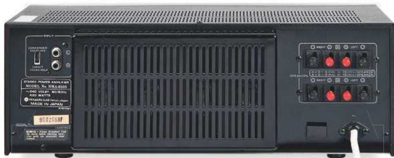
ABOVE: A rear view showing the boxed heatsinking for the hard-working MOSFETs. If using preamps from other brands, use the DC coupling switch (top left) with care
