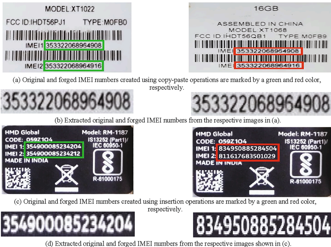
Fig. 1. Examples of copy-paste and insertion operations for creating forged IMEI number images.
