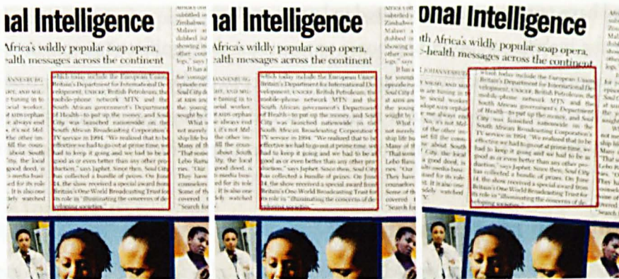
Figure 5.3: A rectangular region shown (a) without skew, (b) with 0.5 degrees of skew and (c) with 5 degrees of skew, all with bounding boxes overlaid.
